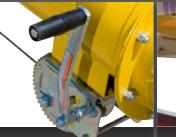
Safety winch with automatic brake Roller with oiled hardwood is sized and geared to match the auger. The strong 1/4" galvanized to raise auger. aircraft type cable has 7000 lbs. break strength.
